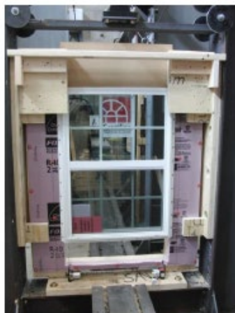
Photo 2: Structural Loading – Fastener/Flange Capacity
