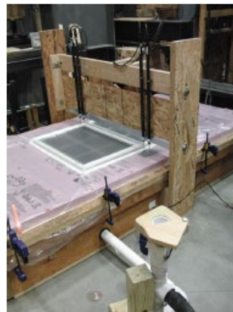
Photo 3: Wind Pressure Loading Test Setup
