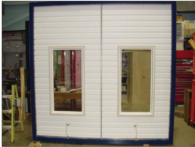
Figure 2. (a) Sample wall-window test assembly; (b) Diagram of wall-window assembly showing locations of wall-window interface details
