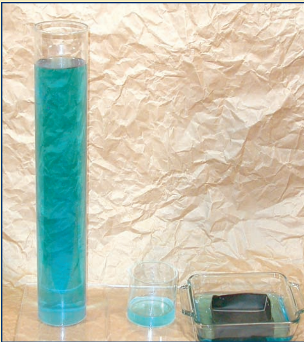
Figure 4. Demonstration of three different hydrostatic heads prescribed by AC38 for water resistance testing of Grade D WRBs. From left to right: 55 cm (AATCC 127), 1 inch (CCMC), and negligible head (ASTM D-779).
