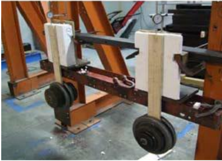
Figure C.2: Typical long-term shear load (creep) test rack set-up
