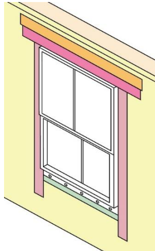
STEP 5: Install External Jamb and Head Flashing & Termination Tape
