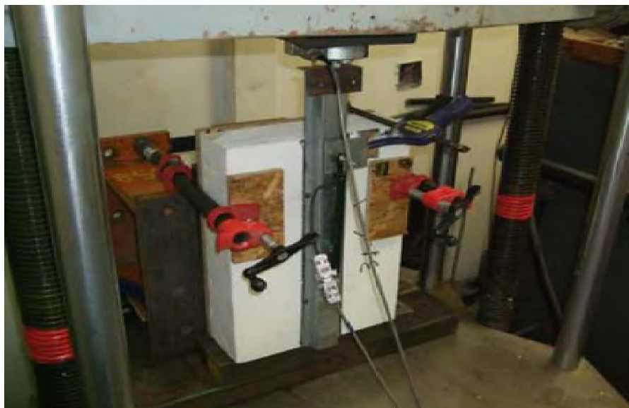
Figure C.1: Typical short-term shear test set-up
