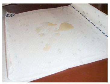
Photograph 12 – Weak Surfactant: Use a teaspoon to drop this weak surfactant solution on the sample. This is Joe Test 3.
