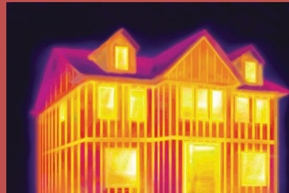
Cavity Insulation Only
