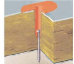
Fig. 2: Version with plastic sleeve and shorter fastener
