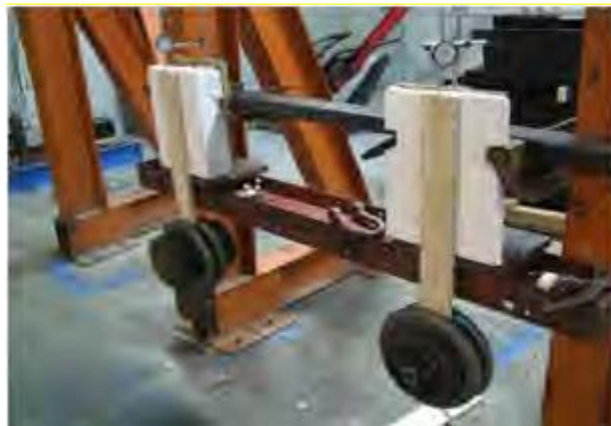
Figure 4. Typical long-term shear load (creep) test set-up
