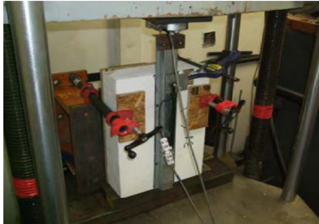
Figure 3. Typical short-term shear test set-up
