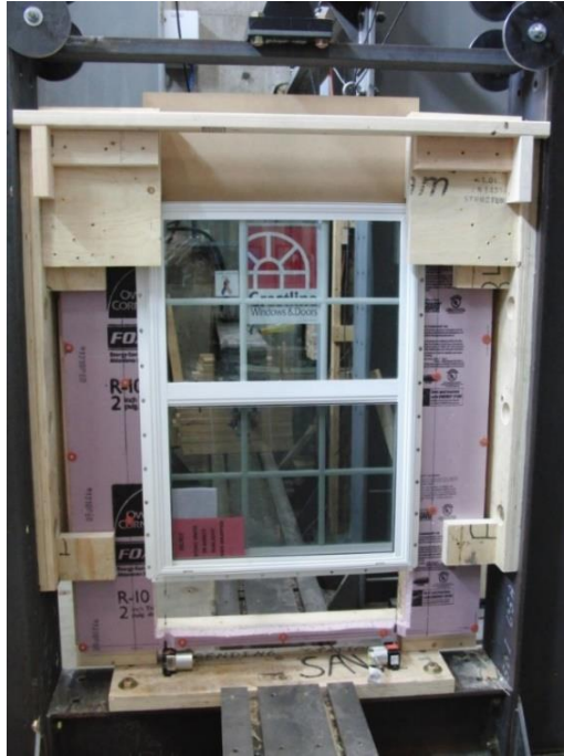
Figure 10. Window installation shear load test set-up.
