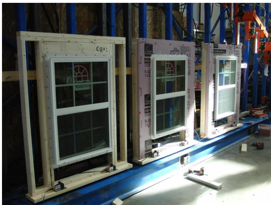
Figure 9. Sustained dead load tests for creep and stability (Qualtim, Inc., 2013). 31
