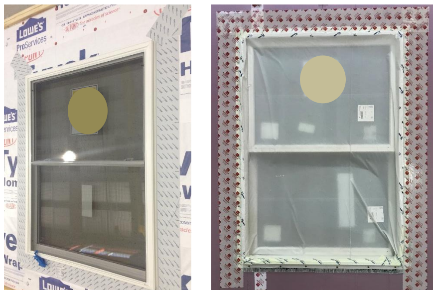
Figure 7. Adhered flashing as installed at window perimeters in test specimens with a building wrap WRB (left) and with FPIS WRB system (right).
