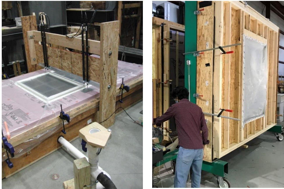
Figure 8. ASTM E330 test apparatuses used to evaluate positive and negative pressure resistance. (LEFT – Specimens A and B; RIGHT – Specimens 1-15 and R1-R3)
