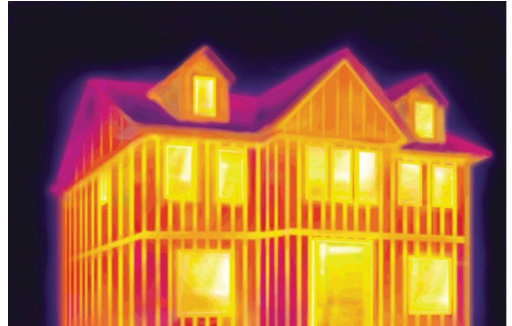
Thermal imaging illustration of unmitigated framing thermal bridges releasing heating energy (no continuous insulation).
