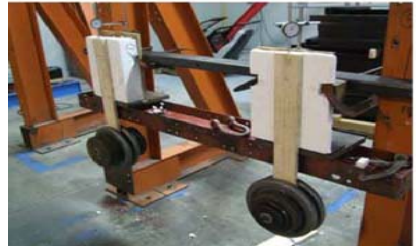
Long-term (sustained) load-deflection test
