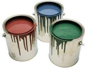
Latex paint film = 3 to 30 perm (primer + 1-2 coats)
