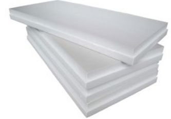
1" thick polystyrene insulation \approx 1 perm to 5 perm No facer. Depending on type/density. Decreases with increased thickness or added facers
