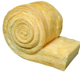
Fiberglass/mineral fiber = 116 perms Batt insulation (without facer), 1” thick
