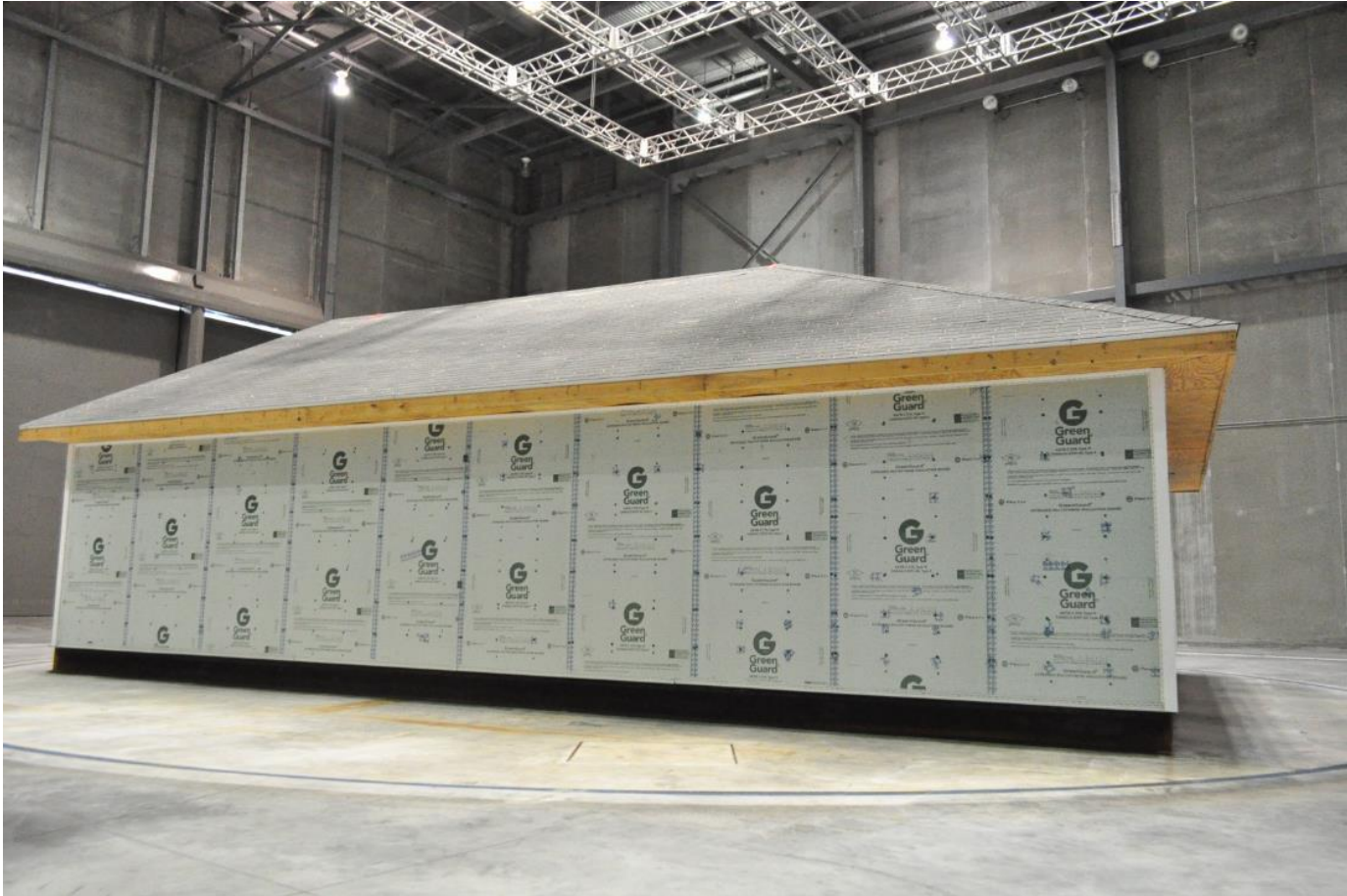
IBHS wind tunnel test (Photo courtesy of Dave Johnston)
