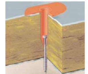
Fig. 2: Version with plastic sleeve and shorter fastener
